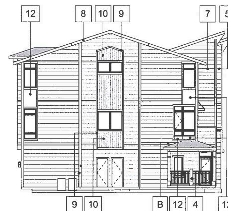
4 West Elevation, Materials 1/8" = 1'-0"
