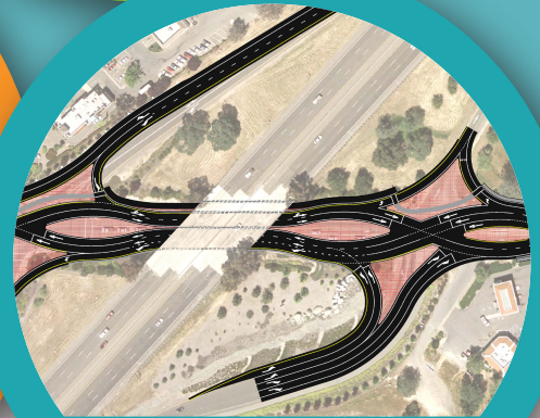
Concept 3: Diverging Diamond Interchange with Adjacent Ped/Bike Undercrossing
