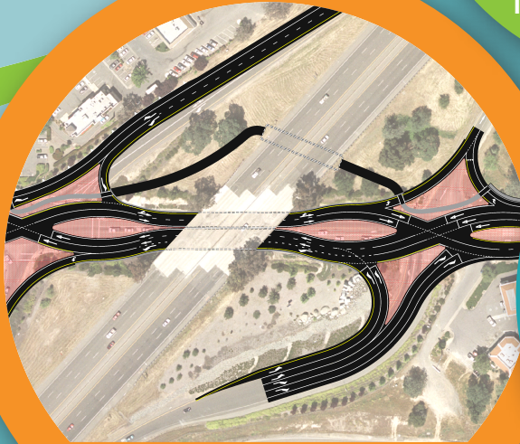
Concept 2: Diverging Diamond Interchange with Separate Ped/Bike Undercrossing
