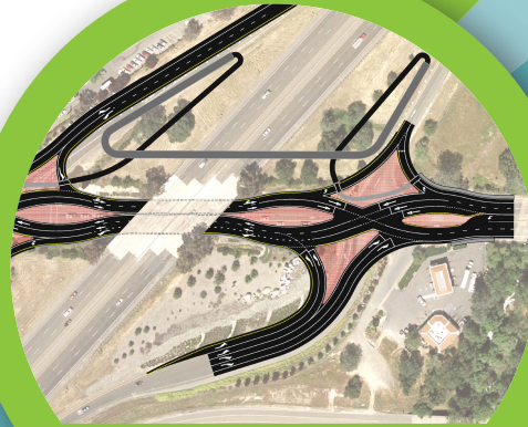
Concept 1: Diverging Diamond Interchange with Infield Ped/Bike Overcrossing
