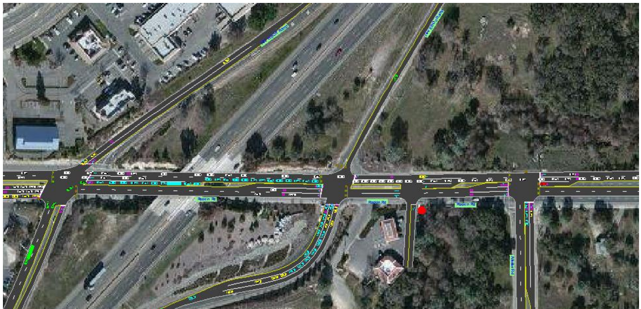
Image shows queue spillback (vehicles in blue) from the I-80 WB on-ramp, which adversely affects the EB ramps and Aguilar Road intersections.
