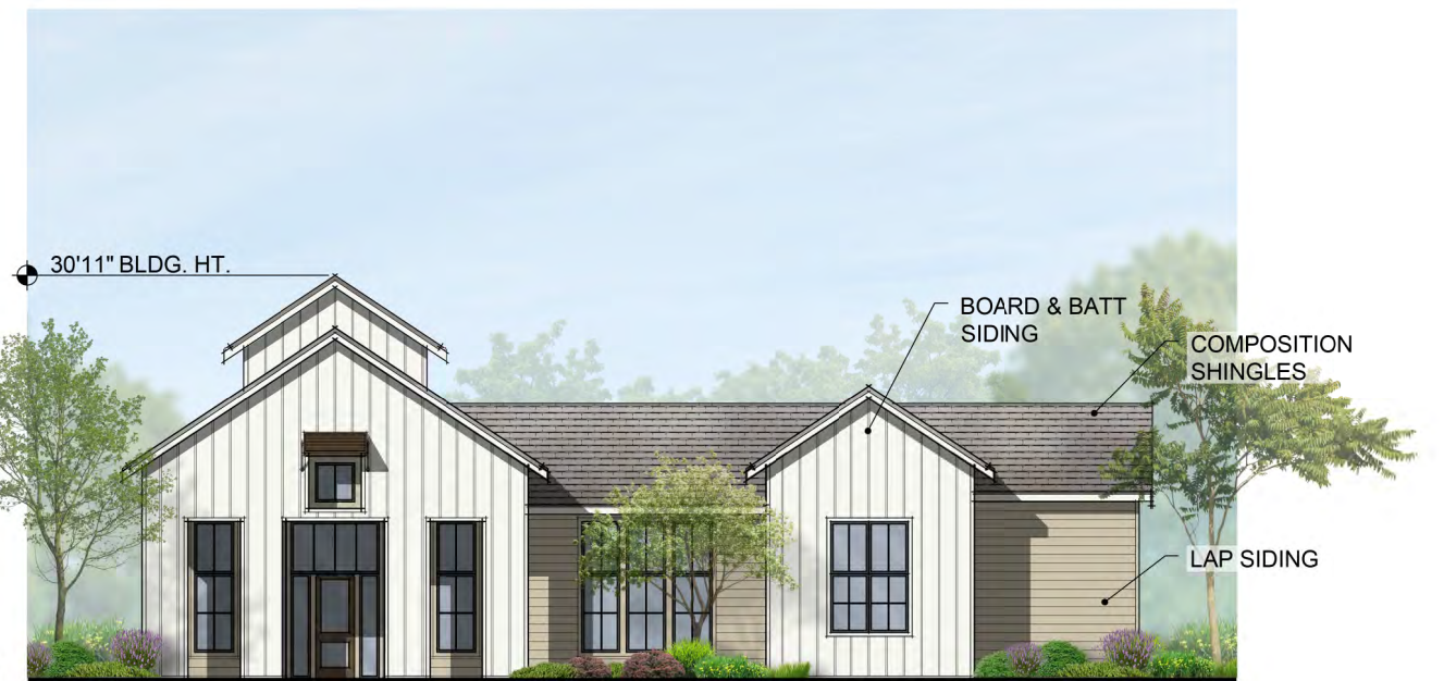
FRONT ELEVATION (SOUTH EAST)
