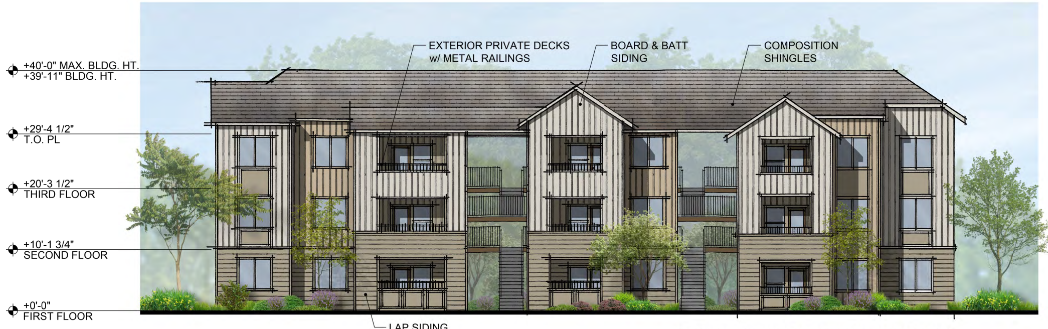
FRONT ELEVATION (NORTH EAST)
