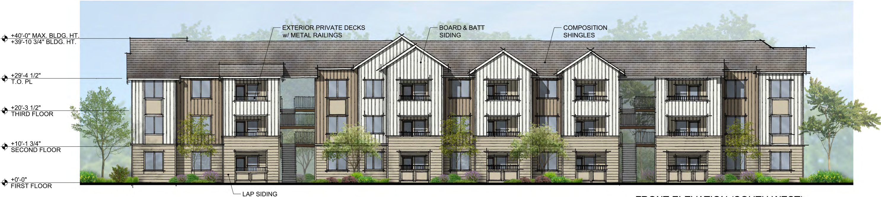
FRONT ELEVATION (SOUTH WEST)
