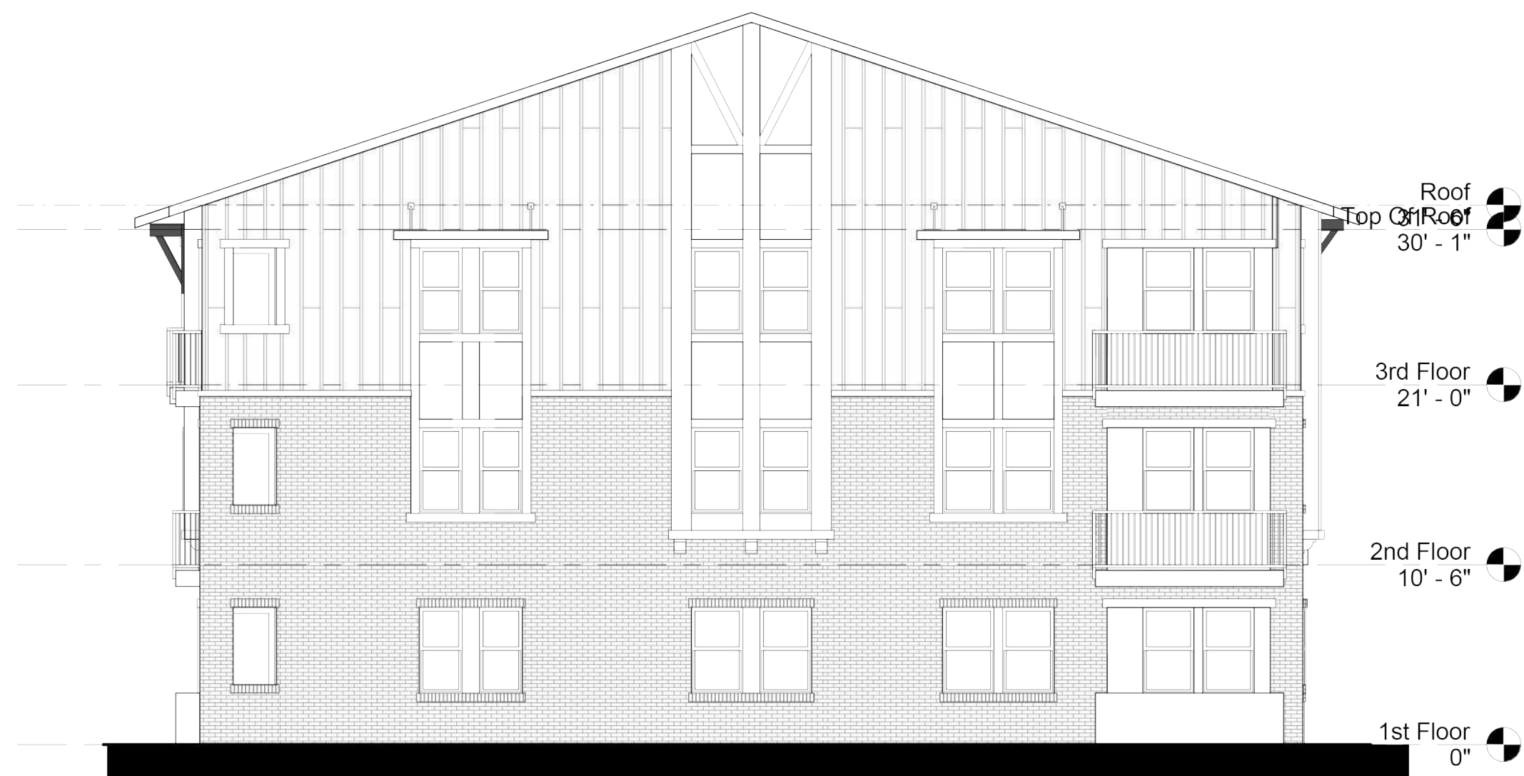
BUILDING 4 - NORTH ELEVATION | 2 1/8" = 1'-0"
