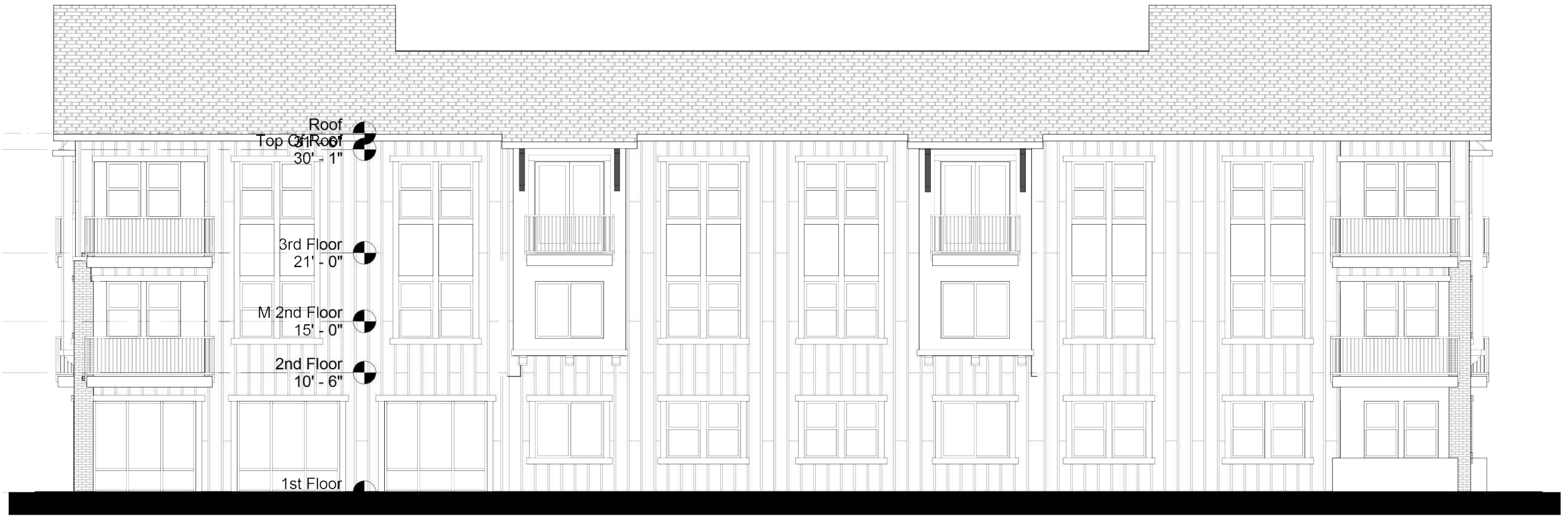
BUILDING 4 - EAST ELEVATION | 3 1/8" = 1'-0"
