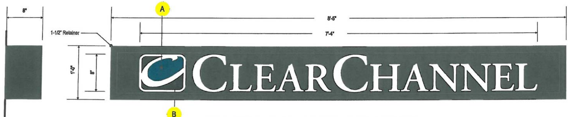
BG-1 S/F ILLUMINATED SIGN CABINETS SCALE: 1" = 1'-0" TWO REQ'D SQUARE FOOTAGE: 8.5
