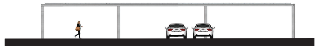
1A. SOLAR CARPORT FRONT ELEVATION
